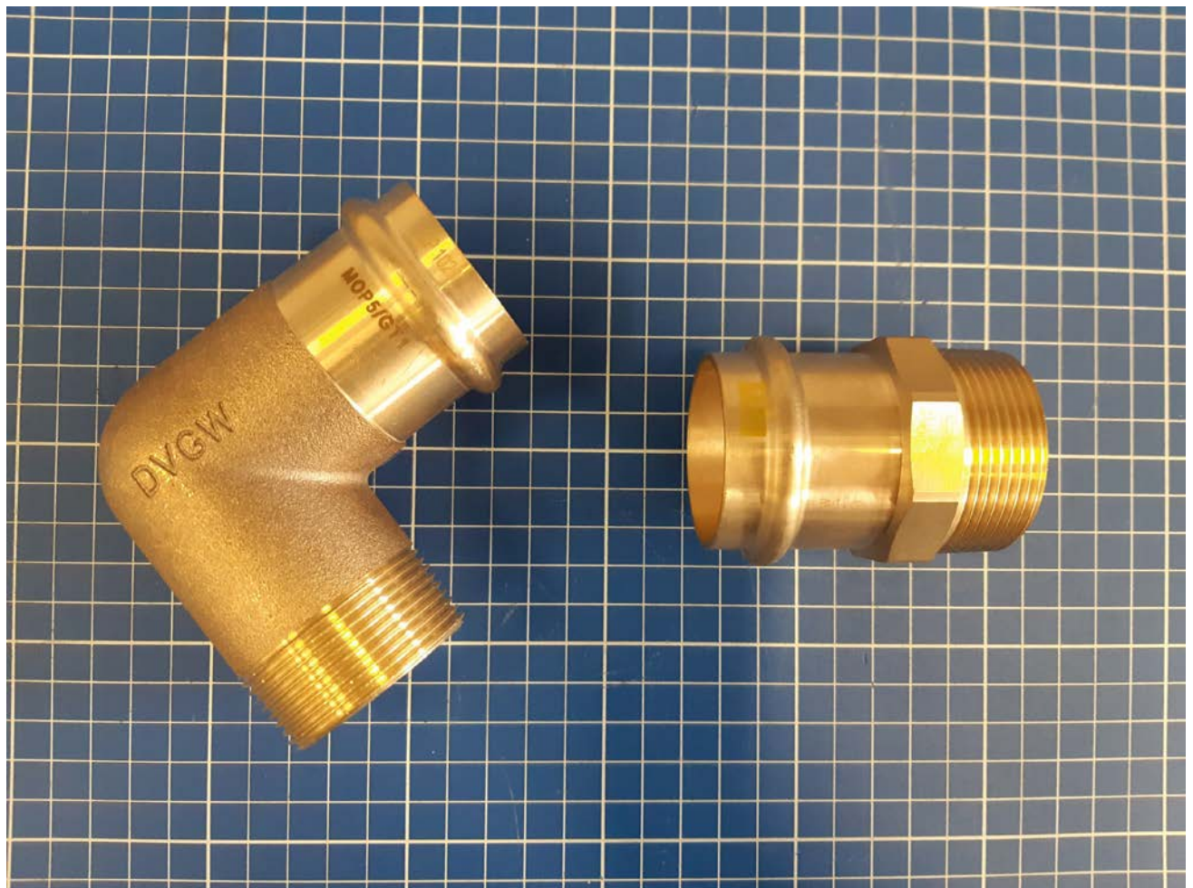
Fig. 1: received test items (red brass articles, DN42)
